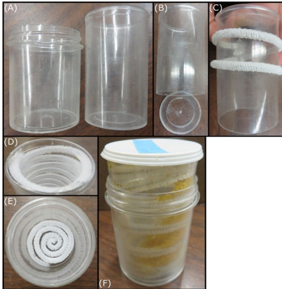
FIGURE 3. Chenille stem feeder design: (A) the 3 oz and 40 dram vials, (B) the bottom of the 40 dram vial sawed off, (C) the chenille stems coiled, (D) the coiled stems glued within the feeder, (E) coiled stem placed at the bottom of the 3 oz vial, (F) 40 dram vial placed into the 3 oz vial with pollen and cap, ready to shake.
